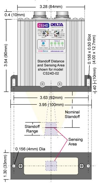
The CS24D is available in several models with a variety of sensing areas and standoff ranges. Standoff ranges include 0.63 to 1.00" (16 to 25mm) and 1.50 to 2.25" (38 to 57mm) shown above.
